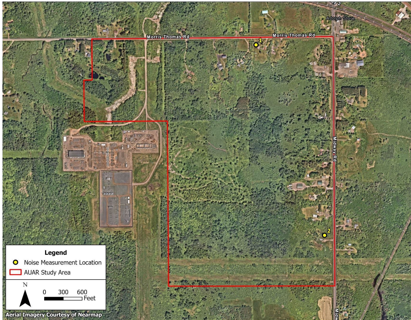
Figure 1. Ambient Noise Measurement Locations
