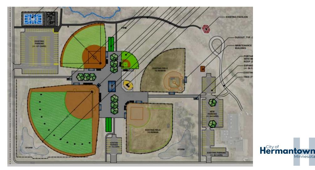
This concept allows for Field 1 to be raised, flipped, and turfed, while upgrading Field 2 and the T-Ball field. Additional parking is added, as well as new playground equipment (that is shaded), a new sport court (basketball) and a new and upgraded skate park. Additionally, this concept fits within the \$3.9 million budget set by the Local Option Sales Tax question on the ballot.
